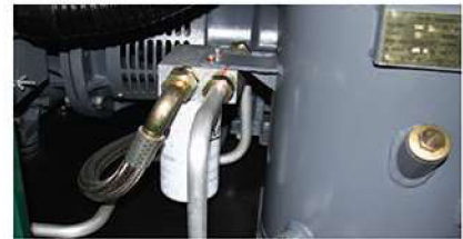
Lubricant filter assembly features a spin-on, full-flow, 12μ, high-efficiency components
