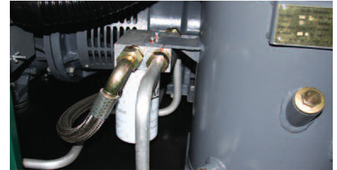
Lubricant filter assembly features a spin-on, full-flow, 12µ, high-efficiency components
